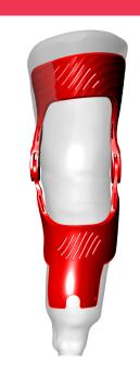
By applying compression during 3D modelization, the perfect fit of the brace eliminates all gaps between the leg and the brace, thus ensuring valgum loads are being transferred to the reinforces uprights of the ExoStab 3D.
