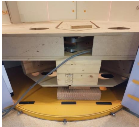
Figure 1: Force platform in the EOS cabinet measures the forces under the studied foot in the middle while the contralateral foot is isolated from the force platform.
